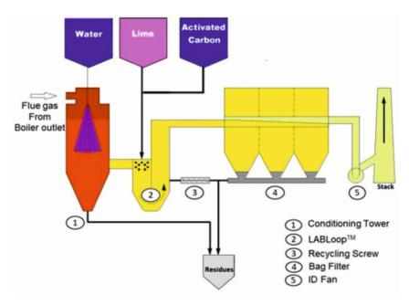
SCHEMATIC OVERVIEW OF SECOLAB™ DRY FGT SYSTEM
